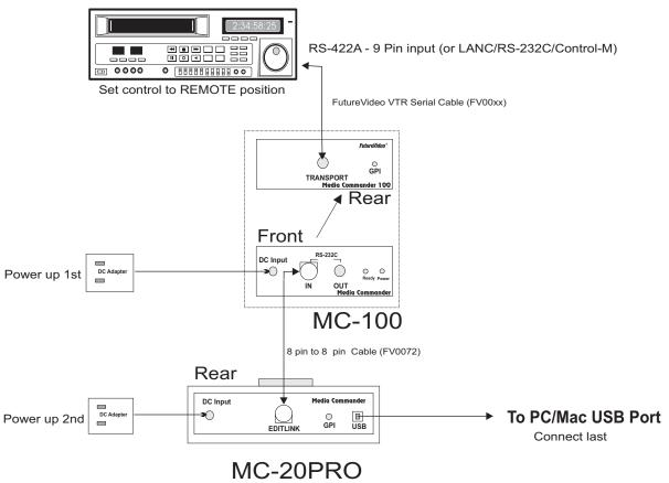
MC-20PRO connection to MC-100 for External Device Control
